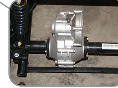
Transaxle: Continuously variable transaxle no noise
