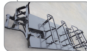
Chassis: High tensile steel welding structure, electrophoresis treatment for the whole chassis enhances the anti-corrosive and anti-rust performance
